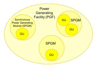
Where generating units are connected via inverters, the inverter rating is deemed to be the generating unit rating.
