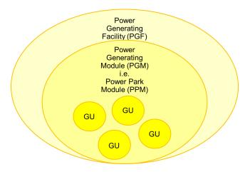
**Synchronous Power Generating Module** – the classification of Type A to D is based on the capacity of **each** Power Generating Module (PGM) in the Power Generating Facility (PFG):
